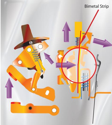
Current flowing through the bimetal strip causes it to heat up. When a certain heat is reached, the strip bends and operates the trip mechanism. The strip is calibrated to start bending when overload amperage is reached. The higher the current flow, the quicker the bimetal trips the breaker.
