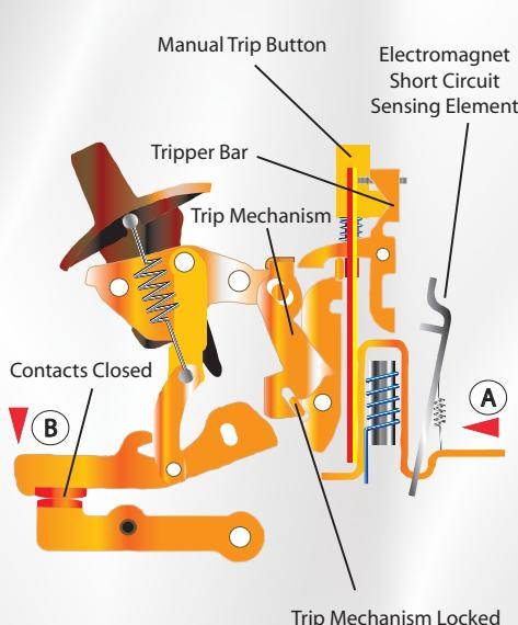
In the "ON" position, as above, the trip mechanism keeps the circuit closed and lets current flow from "A" to "B". The trip mechanism can be engaged manually for overload by thermal sensing and short circuit by an electromagnetic device. There is also a manual trip button.
