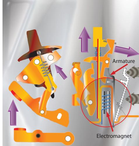
Short circuit protection is provided by the electromagnet. The electromagnet produces a magnetic field sufficient to pull the armature only when overload amperages are reached. Tripping occurs when the armature strikes the trip bar. This cuts current flow and releases the armature.
